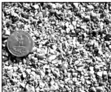
This is a close-up of typical aggregate used as surface topping, showing angularity and size. Photo: RCOC
