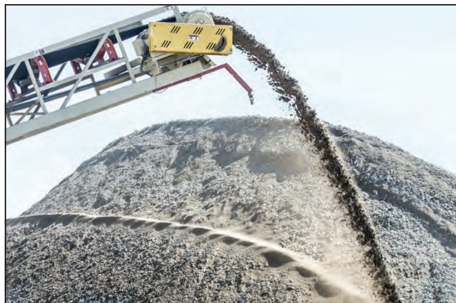
Old concrete is pulverized to be used in the new highway. Photo: Tim Jagielo
