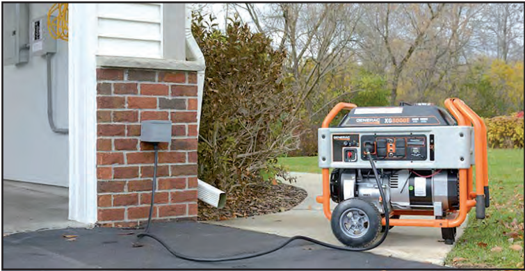
A generator must not only be outside the home — the exhaust cannot be leaking into the home as it runs. Photo: www.norwall.com
