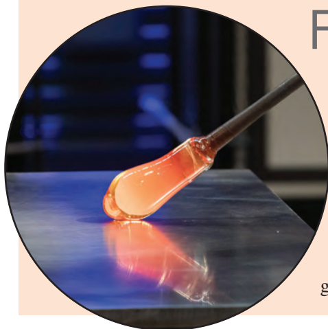
(Above) Flint Institute of Arts Instructor/demonstrator Andy Koupal forms the glass with wet newspaper as technician Benjamin Ewing blows to expand it. (Below) The molten glass is rolled along the stainless steel marver table to begin shaping it.
