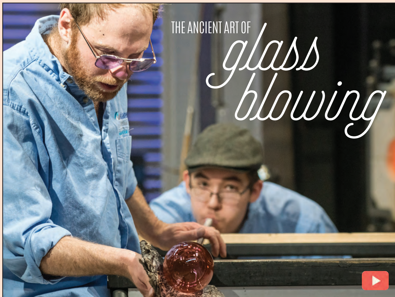
(Above) Flint Institute of Arts Instructor/demonstrator Andy Koupal forms the glass with wet newspaper as technician Benjamin Ewing blows to expand it. (Below) The molten glass is rolled along the stainless steel marver table to begin shaping it.
