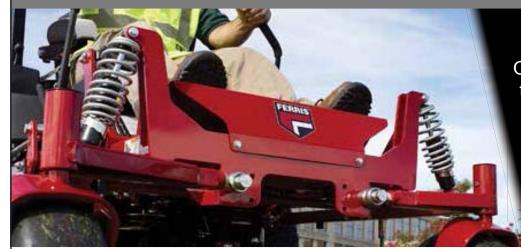
Our patented suspension systems are engineered to provide you with a smooth ride on uneven turf. The deck of the mower works in conjunction with the suspension system to provide a consistent quality of cut. This system minimizes shock to the chassis, resulting in stability, speed and increased productivity.
